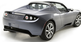
Figure 11. Good: The Tesla Roadster electric car. Energy consumption: 15 kWh per 100 km . www.teslamotors.com .
